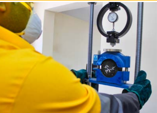
THE MARSHALL STABILITY AND FLOW TEST
